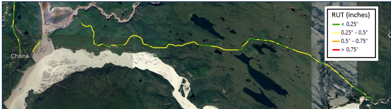
Figure 4-9. Roadway Rutting in the Study Corridor, MP 3 to MP 17
