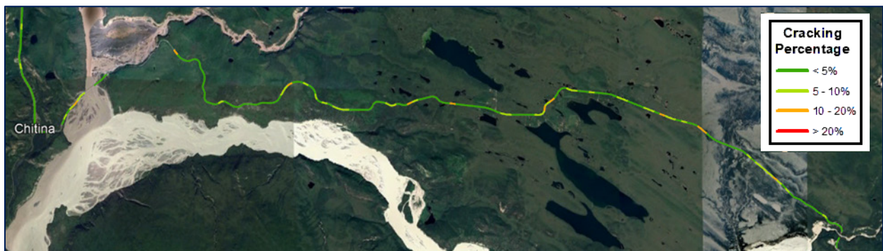
Figure 4-10. Roadway Cracking in the Study Corridor, MP 3 to MP 17
