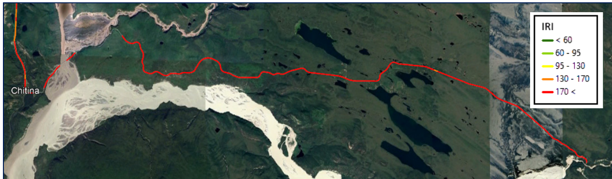
Figure 4-11. Roadway Roughness in the Study Corridor, MP 3 to MP 17
